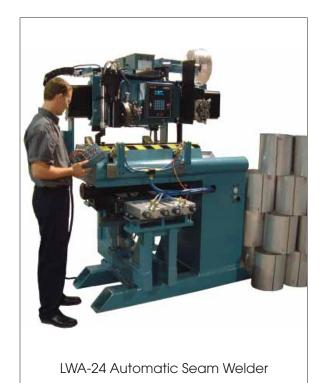
To speed up the loading and unloading process, automatic seam welders are usually manufactured without a mandrel latch and with a larger diameter mandrel than normal. For special applications, especially where it is necessary to accommodate smaller diameter parts, a mandrel latch is available.
